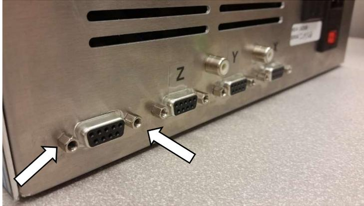
7. Use the 2 included screws to attach the 4<sup>th</sup> axis driver board to the aluminum heat sink using the 2 screw holes. Once these screws are in place, fully tighten the 2 screws and the 2 hex bolts attaching the 4<sup>th</sup> axis driver board to the back of the HD4 controller. (Optional: add a dab of heat transfer compound in between the driver board and heat sink)
